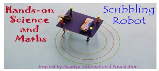
IN THIS EXPERIMENT THE TABLE TOP HAS A TOY MOTOR WITH AN OFF-CENTER SHAFT. THE LEGS OF THE TABLE ARE 4 DIFFERENT COLOUR SKETCH PENS.
