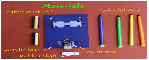
MATERIALS: A RECTANGULAR ACRYLIC SHEET WITH 4 HOLES FOUR COLOR SKETCH PENS TOY MOTOR WITH BATTERY PACK RUBBER SHAFT WHITE PAPER
