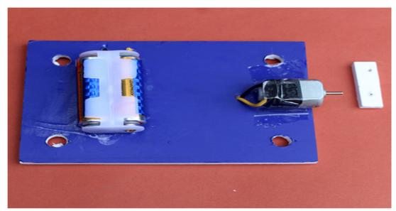
ON THE ACRYLIC SHEET IS MOUNTED A TOY MOTOR AND A BATTERY PACK. THE RUBBER PIECE WILL BE AN OFF-CENTER SHAFT.
